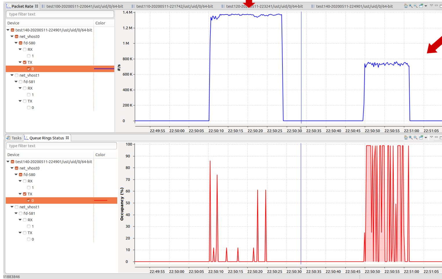
Figure : Host is sending packets to the guest. (UP) Rate of MBuffer enqueueing. (DOWN) Percentage of TX queue occupancy.
