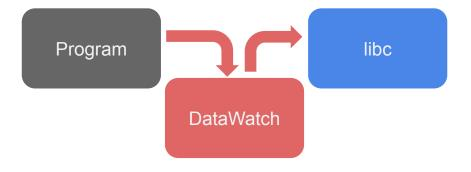
Each pointer resolution now raises a segmentation fault, which is handled by DataWatch. If the dereference is within bounds, it corrects the address and sends back the value.
