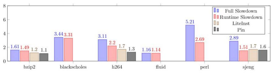
Instrumentation and runtime overhead of a procedure counter on different applications of the SPEC suite, relative to uninstrumented execution time.
